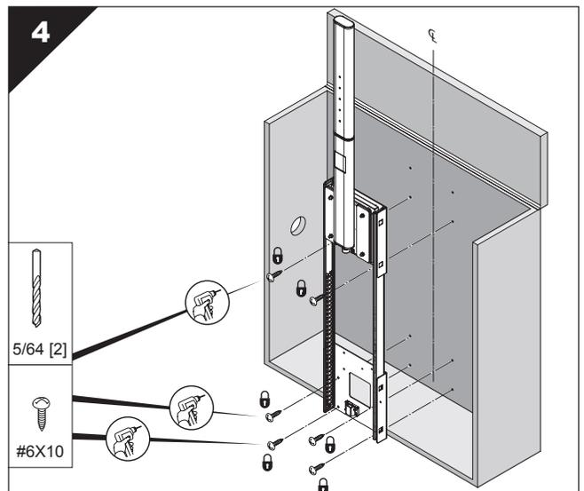
Lower the lift (see Figure 5) to the mid-travel point to expose the final two mounting holes. Install two #6 X 10 screws and secure.
