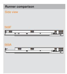
**NOTE:** Material thickness may vary. Inside drawer width **must** equal opening width minus **49** for TANDEM to align and function properly.
